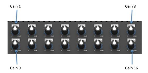
As these are analogue gain, the gain setting will remain unchanged regardless of the scene change.
